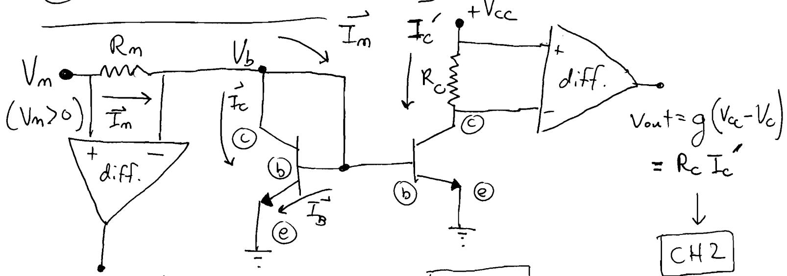
$$V_{out} = g(V_m - V_b) = I_m R_m = \boxed{CH1}$$
