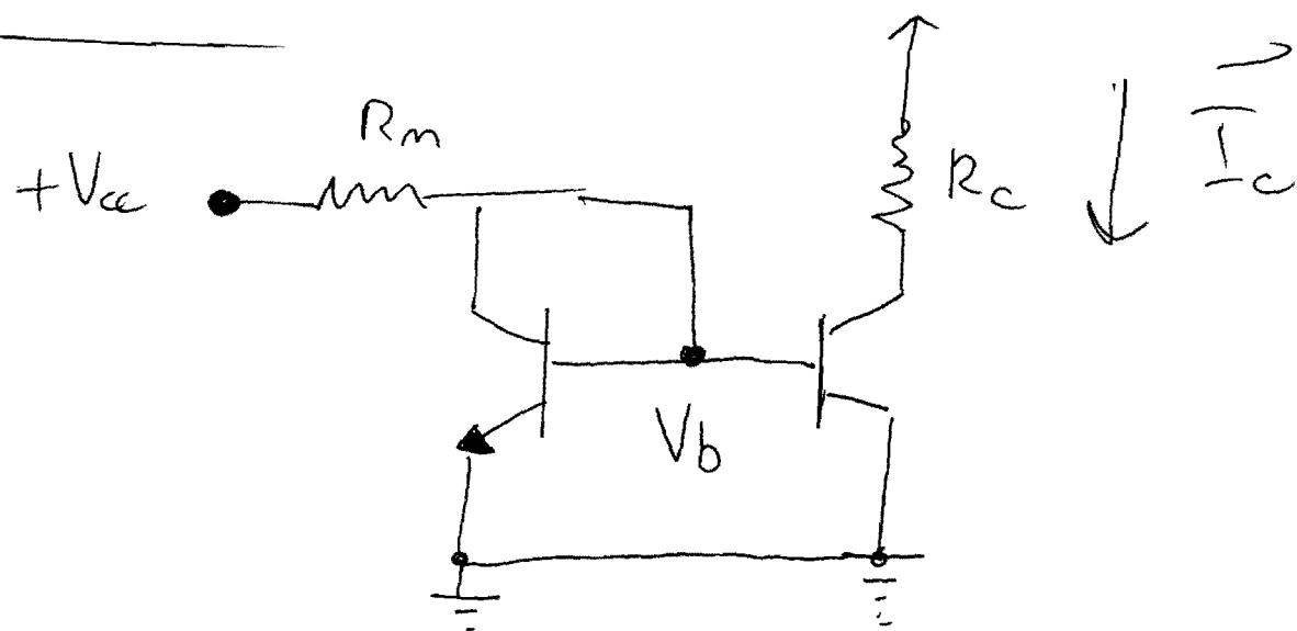
The whole point of the current mirror is to establish a constant  $V_b$  (shown on page ②), this constant  $V_b$  creates a constant  $\bar{I}_c$ . Because  $\bar{I}_c$  is held constant any resistor (or circuit) will adjust its potential drop to maintain constant current.
